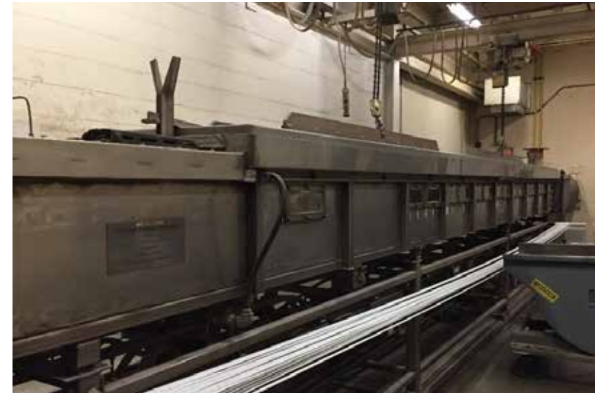
Image of Steiner Tunnel at UL LLC
